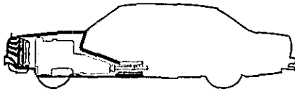
Fig. 4 - Engine compartment encapsulation Basic sketch of vehicle-supported capsule
